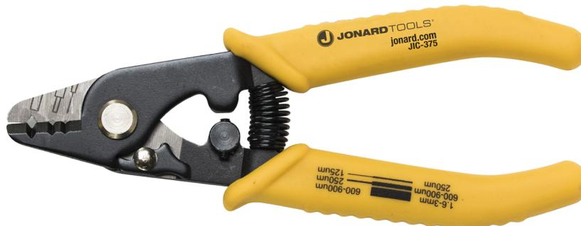
**JIC-375 Fiber Optic Stripper Three Hole:** This innovative new three hole model performs all common fiber stripping functions. Strips the 1.6-3 mm fiber jacket down to the 600 - 900 micron buffer coating. The second hole strips the 900 micron buffer coating down to the 250 micron coating and the third hole is used to strip the 250 micron cable down to the glass fiber without nicks or scratches.
