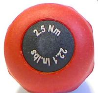
The fixed pre set Torque size can be found on the butt of the handle.
