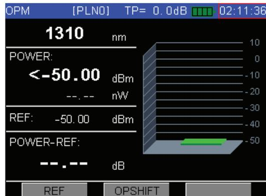
Figure 8: Optical Power Meter Function
