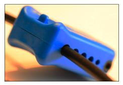
Pull the tool towards the end of the cable and the PE jacket is then slit on 2 sides enabling easy removal of the jacket and provides exposure of the indoor part of the cable.
