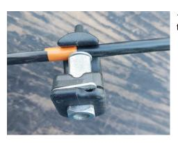
1. Remove around 1m from the end of the cable. Mark 1,5 meter and remove the cable sheet with suitable stripper
