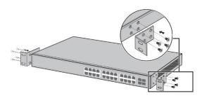
4. Put PoE switch on the appropriate location of the rack, crutch by bracket; using the L-shaped bracket to fix the two sides of rack with screw, make sure PoE switch is installed on the rack smooth and steady.
